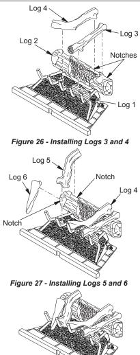
Figure 28 - Logs Installed for M36, M36P, VM36 and VM36P Models
